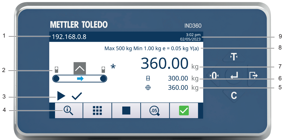
Display in In-motion weighing mode
