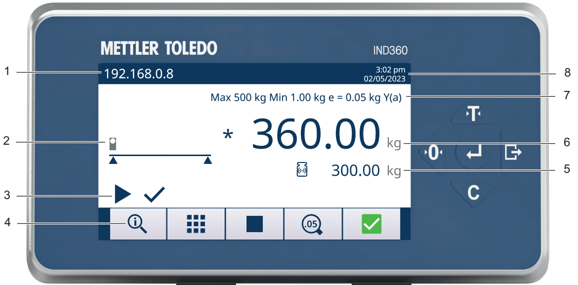
Display in Static weighing mode
